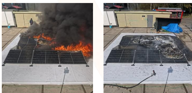
Fig. 3: Fire behaviour of BAPV on a flat roof with A1-insulation, during and after extinguishment.
